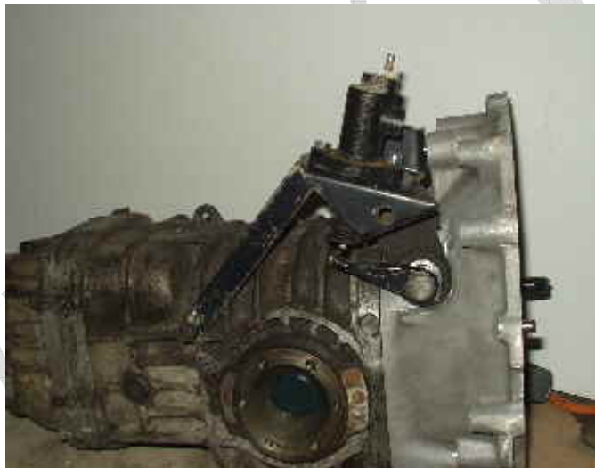
RJES Bell Housing Mounted to VW Gearbox
