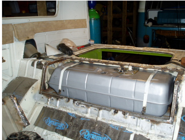
Subaru pump and tank internals grafted into a Bay fuel tank
